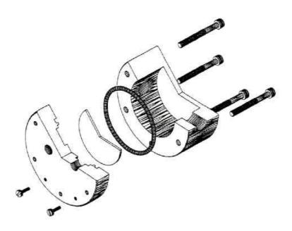
The design facilities large filter surface combined with small volume and is ideal for use with Wet Chemistry analysis. The filter element is easy accessable for cleaning and replacement.
