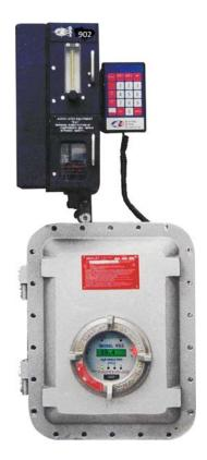
The model 902 H<sub>2</sub>S / Total Sulphur analyzer from Galvanic Applied Sciences Inc. is designed to measure H<sub>2</sub>S in gaseous streams. The 902 detection system is based on the lead acetate tape method. With the optional total sulphur furnace, the unit can measure alternate readings between H<sub>2</sub>S and total sulphur. The 902 is capable of measuring up to eight streams.
