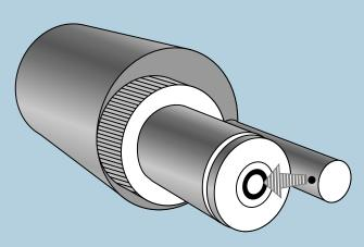
A blast of air keeps the Auto-Clean sensor clean.
