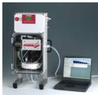
For online condition monitoring, the PAMAS WaterViewer can be fixed at the wall. Equipped with an aluminium mounting rack, it can also be used for on-site measurements.
