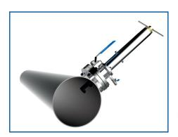
The i::scan in-pipe fixture allows for measurement directly in the medium without any bypasses. The in-pipe fixture has been designed and tested to work with a pressure of up to 10 bar. It contains a shut off valve that that enables to remove the sensor for maintenance without interfering with the flow of the mains.
